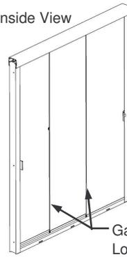
**Step 7.** Install Gap Seals onto the inside edges of Glass Panels, with the soft finger seal reaching toward the outside of the unit.
